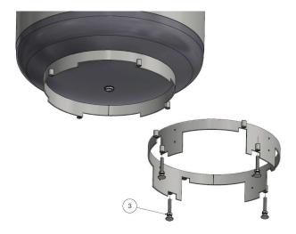
3. Detach the levelling feet from the lower framework.
