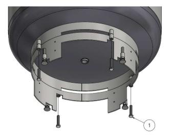
1. Detach the lower framework by loosening the bolts.
