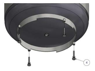
4. Screw the legs into place on the framework that was left on the bottom of the accumulator.
