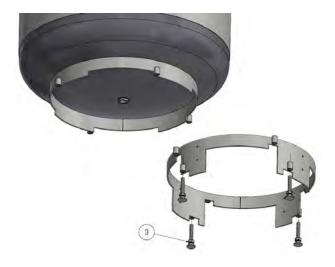
3. Remove the adjustment feet from the lower frame.
