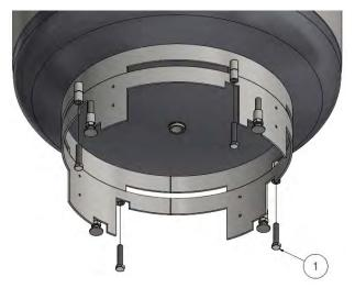
1. Remove the lower frame from the upper frame by loosening the bolts.
