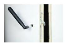
The storage tanks are equipped with removable insulation as standard. The insulation blocks are easy to remove and replace. The insulation blocks can be removed by opening the quick-release fasteners with the handle supplied with the storage tank.
