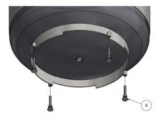
4. Screw the adjustment feet to the frame remaining at the bottom of the storage tank.
